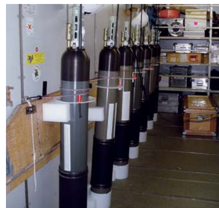
NEMO floats being prepared for deployment (The current version can reach a maximum depth of 2000 m)
