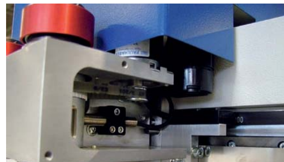
Compact tool head with four motors for two-axis control. The drive is hidden under the cover to save space
