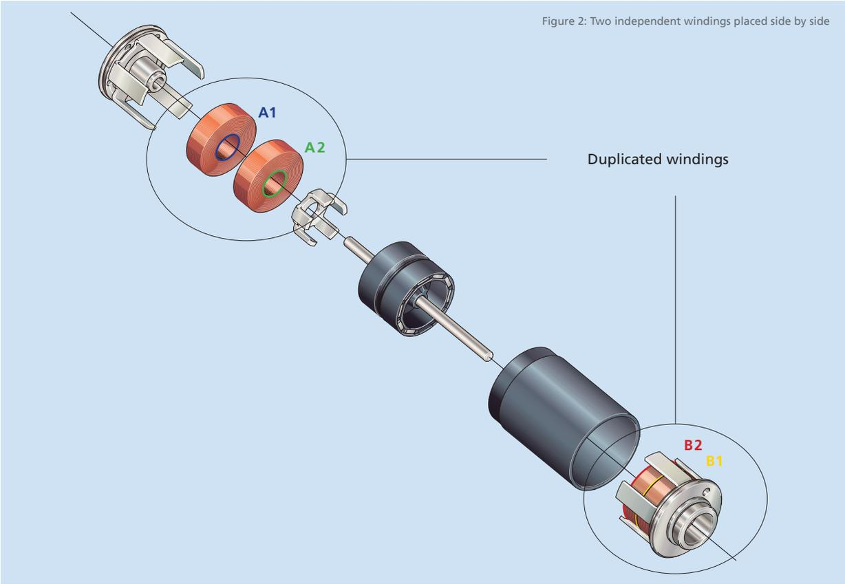
Figure 2: Two independent windings placed side by side
