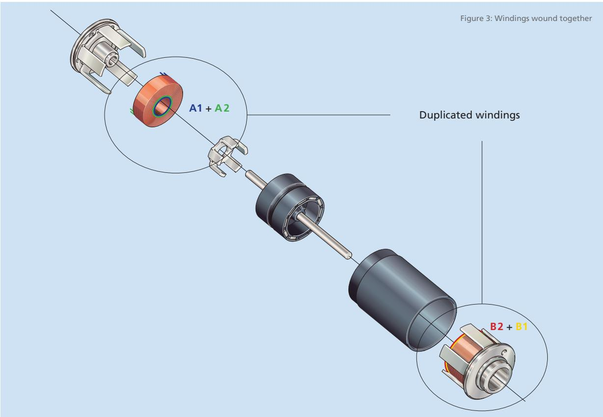
Figure 3: Windings wound together
