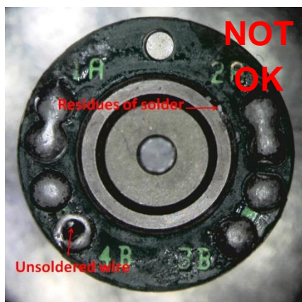
Figure 4 : Good and bad examples of a solder on various PRECISTEP® stepper motors.
