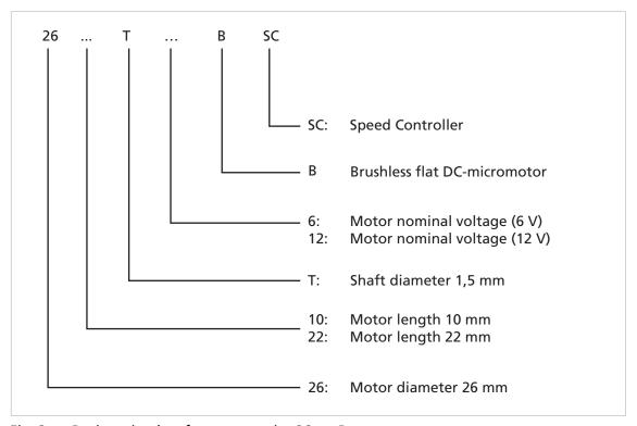
Fig. 3: Designation key for motor series 26xx...B
