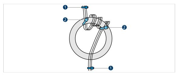
Fig. 19: Coiling ferrite ring
