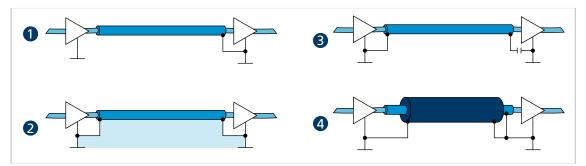
Fig. 15: Various possibilities for the shield connection
