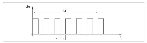
Fig. 25: Signal structure of frequency output
