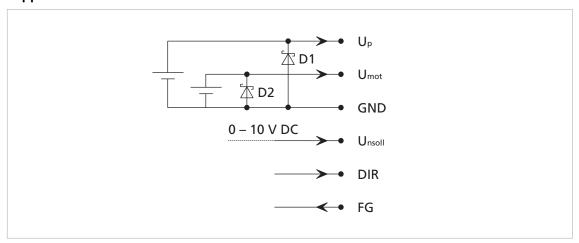
Fig. 9: EMC suppressor circuit with suppressor diodes
