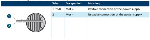
Tab. 8: Electrical data – motor connection (SCDC)
