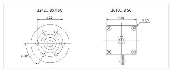
Fig. 7: Comparison of round flange and quadratic flange
