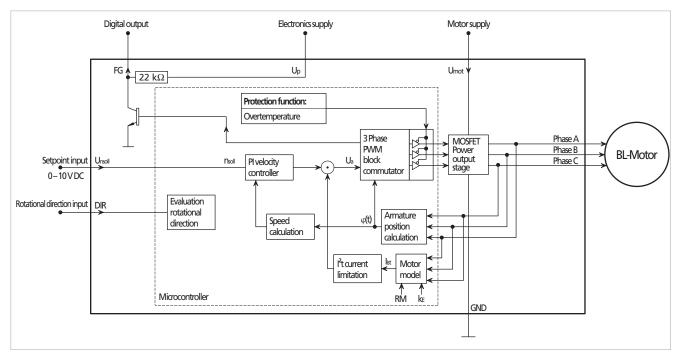
Fig. 22: Block diagram of a BL motor without Hall sensors
