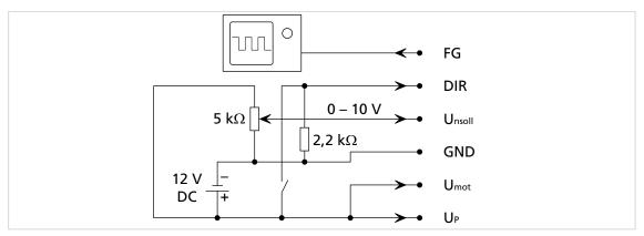
Fig. 10: Normal operation (speed set value specification by U<sub>nsoll</sub>)
