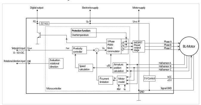
Fig. 20: Block diagram of a BL motor with digital Hall sensors
