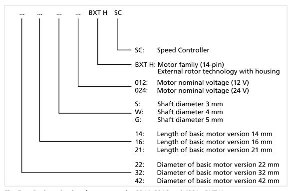
Fig. 5: Designation key for motor series 2214, 3216 and 4221...BXT H
