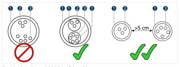
Fig. 14: Grouping and shielding of the cables
