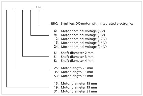
Fig. 4: Designation key for motor series 1525, 1935 and 3153...BRC
