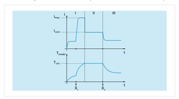
Fig. 27: Example of I<sup>2</sup>t current limitation
