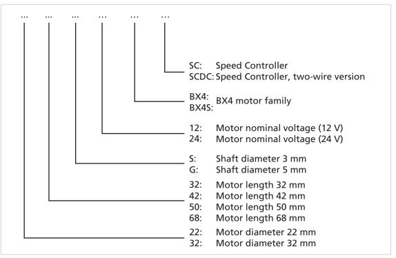
Fig. 2: Designation key for motor series 22xx and 32xx...BX4
