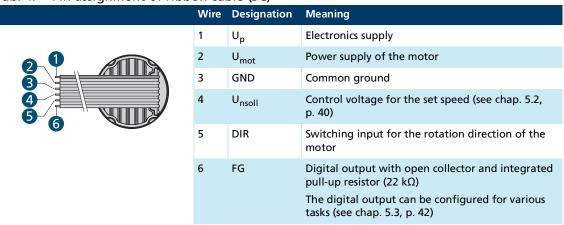
Tab. 5: Electrical data – motor connections on motor series 22xx BX4(S) SC
