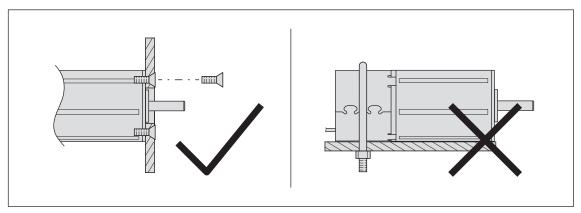
Fig. 6: Mounting example – 22xxBX4 SC series
