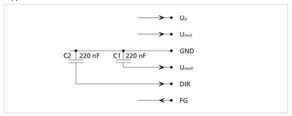
Fig. 8: EMC suppressor circuit with ceramic capacitors
