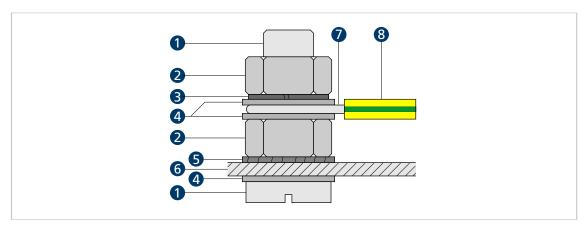
Fig. 17: Shield connection with cable lug
