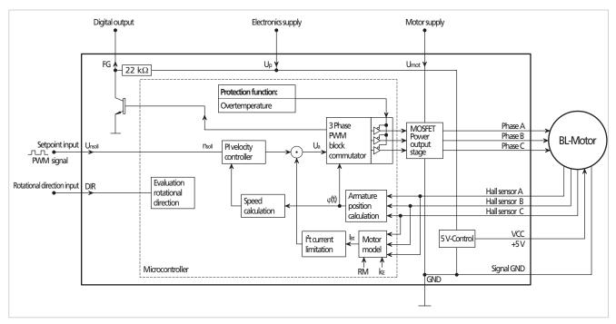
Fig. 24: Block diagram of a motor with integrated SC in PWM mode
