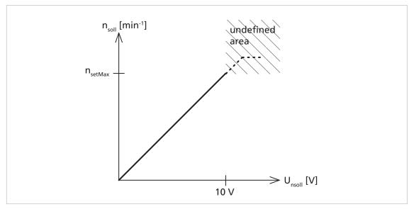
Fig. 23: Set value determination for speed controller
