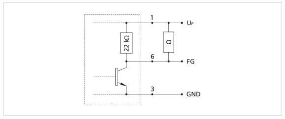
Fig. 26: Connection of an additional pull-up resistor
