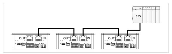
Fig. 2: Connection to the EtherCAT network
