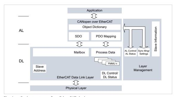
Fig. 1: Basic structure of an EtherCAT device
