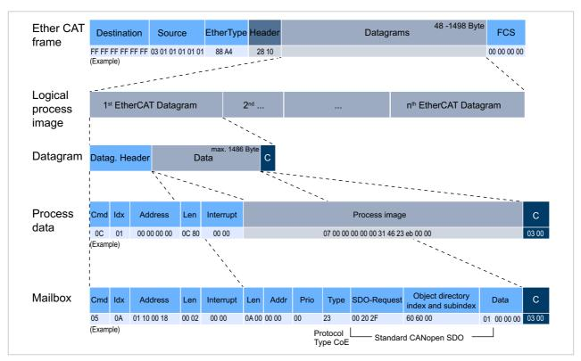
Fig. 4: Frame structure
