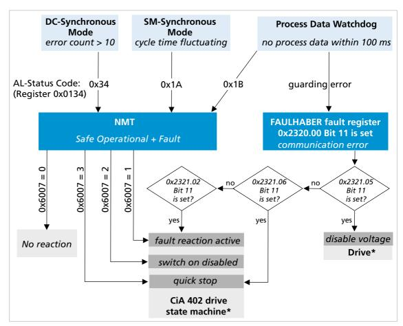
Fig. 7: Mechanisms of error monitoring
