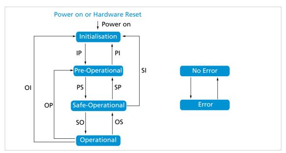
Fig. 6: EtherCAT state machine
