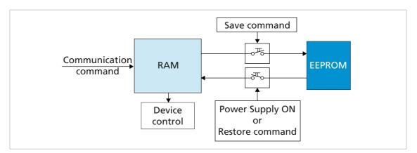
Fig. 8: Saving and restoring parameters
