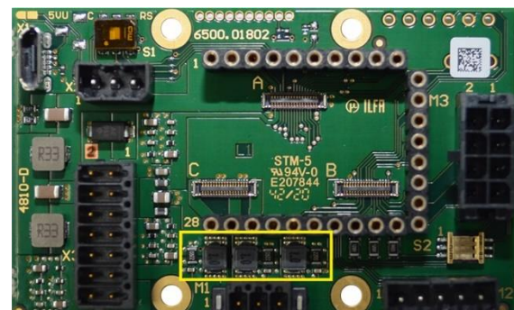
Figure 14: Motor phase filters on motherboard 6500.01802
