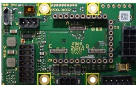
Figure 9: Motherboard 6500.01802 with mounting holes and EGND pads
