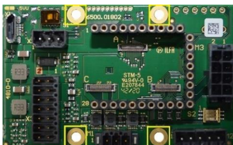
Figure 9: Motherboard 6500.01802 with mounting holes and EGND pads
