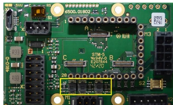
Figure 14: Motor phase filters on motherboard 6500.01802
